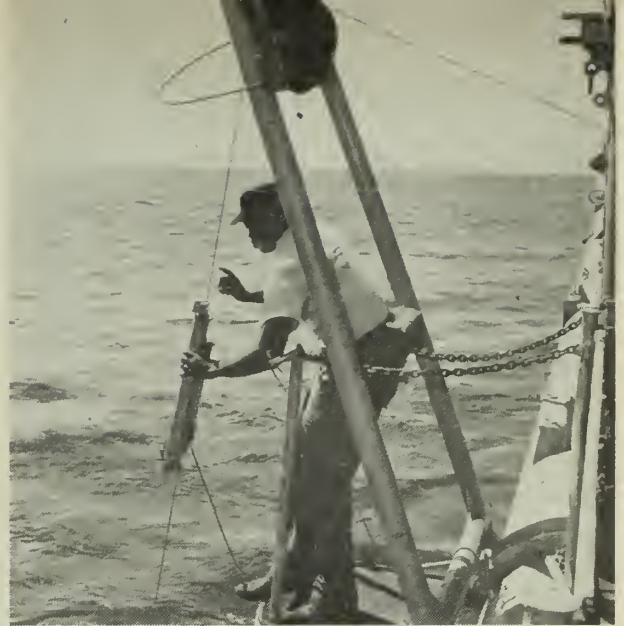
GOING DOWN—Member USS Rehoboth (AGS 50) starts Nansen bottle into sea for temperature and salinity tests.
